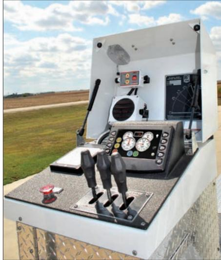
**AL-11 AERIAL LOGIC:** A totally integrated system that provides instant feedback on a ladder's extension, location, retraction, angle, load and breathing air system status, as well as J1939 engine information.
