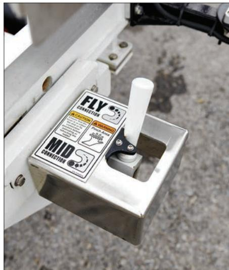
**WATERWAY CONTROLS:** Repositioning the waterway can be done easily with the flip of a mechanical lever. Available on Ladder Tower aerials.
