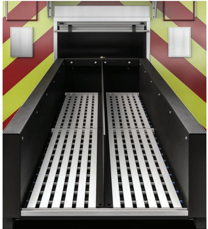
**ERGONOMIC HOSE LOAD (EHL):** *Our patented, heavy-duty, electric/hydraulic hose loader option improves crew safety by placing a maximum of 1,000 feet of 5" LDH within a firefighter's reach, eliminating climbs on a wet or slippery apparatus to reload hose. Available on Smeal Rear Mount aerials.*
