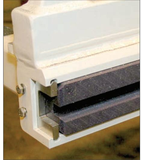
**LADDER SLIDE PADS:** Load Transfer Pads and Front, Rear, and Side Slide Pads reduce friction and ensure smooth ladder operation. Slide pads are also designed with accessibility in mind for easy inspection and replacement.
