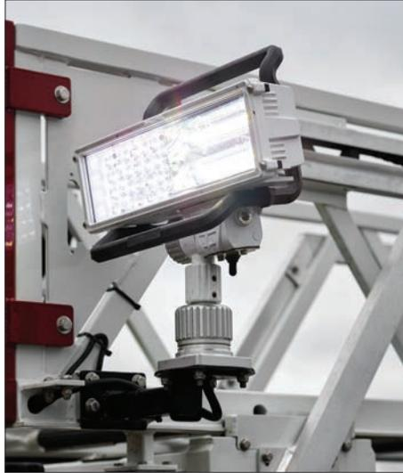
**LED LIGHTING:** All warning and compartment lights are LEDs for long service life, high visibility, and extreme energy savings.
