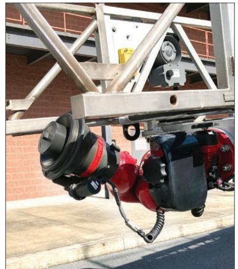
**WATER MONITOR:** When positioned at the tip, the water monitor can be set to reach 30° higher than the elevation of the ladder.
