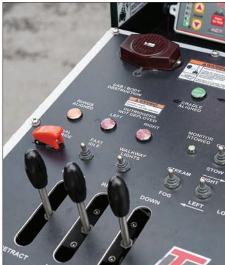
**SPARTAN SELF-LEVELING SYSTEM (SSL):** At the push of a button, after the outriggers are deployed the truck is automatically leveled. The optional SSL system also stows the outriggers at the touch of a button. Available on Smeal aerials.
