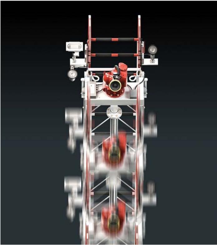
**POSITIONAL WATERWAY:** *Never climb another ladder just to reposition the master stream. Our patented electric positional waterway lets the operator position the waterway to either Rescue or Water Tower mode with a simple one-step procedure from the turntable. Available on Smeal aerials.*
